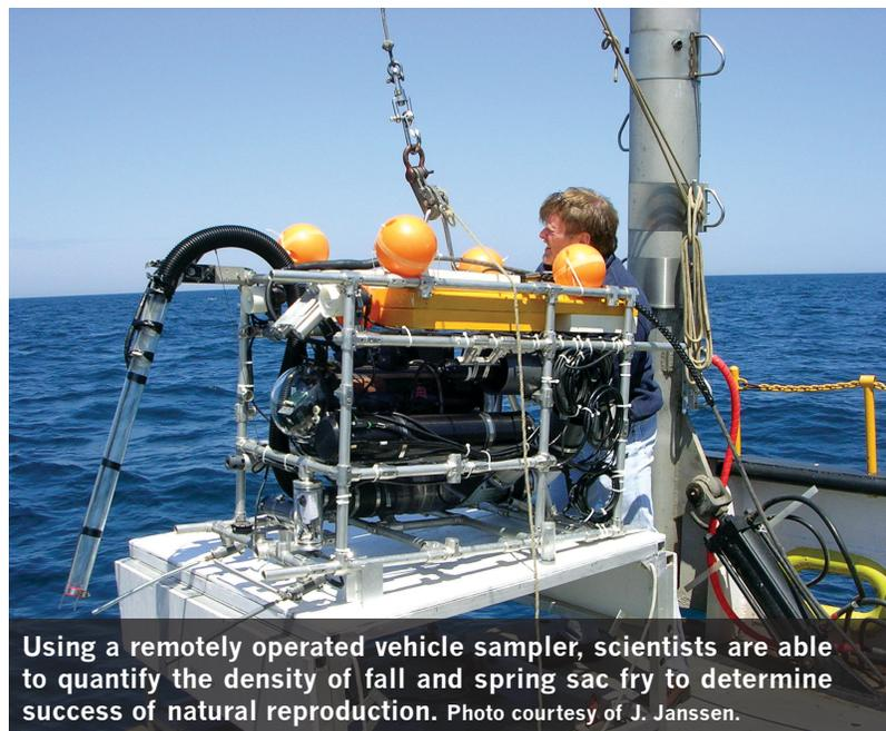
Using a remotely operated vehicle sampler, scientists are able to quantify the density of fall and spring sac fry to determine success of natural reproduction. Photo courtesy of J. Janssen.
