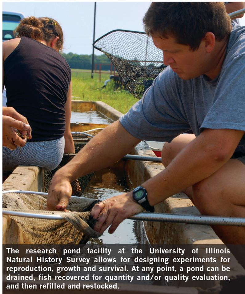
The research pond facility at the University of Illinois Natural History Survey allows for designing experiments for reproduction, growth and survival. At any point, a pond can be drained, fish recovered for quantity and/or quality evaluation, and then refilled and restocked.
